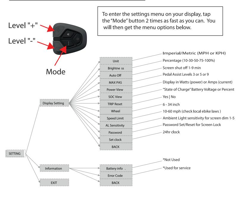
The Level + and Level - buttons are used to navigate the menu, as well as to highlight between options within each menu. The Mode button is used to select.
